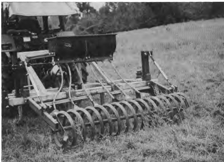
A subsoil plow with ring roller and seedbox. The chisel (or Yeomans plow).
