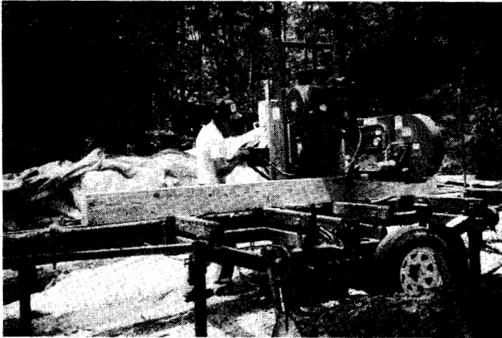
Jon Tiemann cuts pine logs felled nearby on his portable band saw
