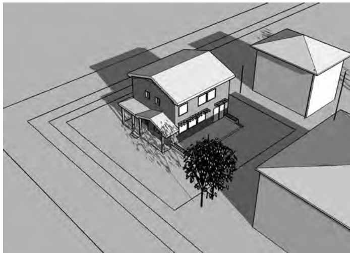
3d SketchUp model with neighboring buildings and trees recreated from Solar Pathfinder data in the previous photo. I used a computer model to determine how far to elevate the floor of the Passive House to ensure that windows were not shaded in mid-day on the shortest day of winter. Drawing by CASnyder.
